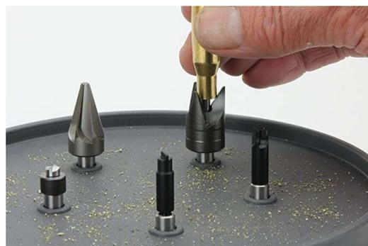
**Fig. 12** The adapting case neck for seating a bullet
